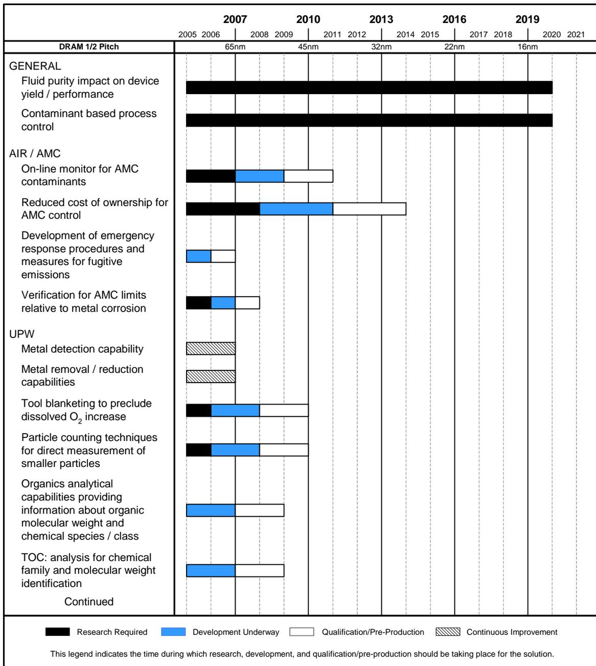
Figure 105 Wafer Environmental and Contamination Control Potential Solutions
