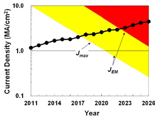
Figure MM10: Evolution of  $J_{max}$  (from device performance) and  $J_{EM}$  (from targeted lifetime).
