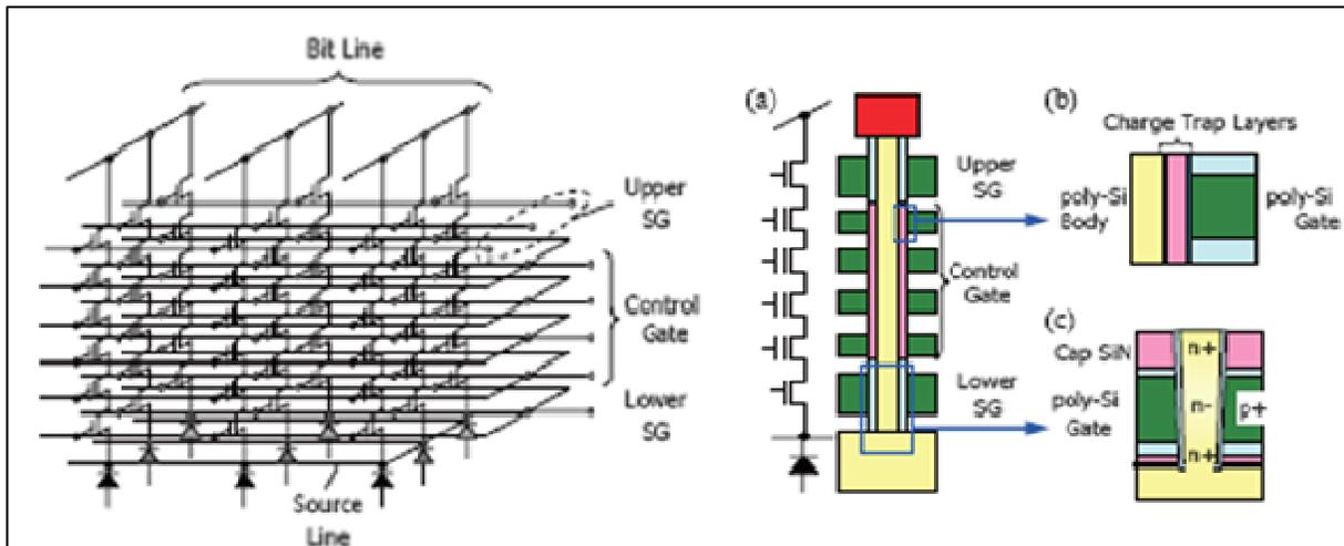
Figure MM7: (left) A 3D NAND array based on a vertical channel architecture [1]. (right) BiCS (Bit Cost Scalable) – a 3D NAND structure using a punch and plug process [1].
