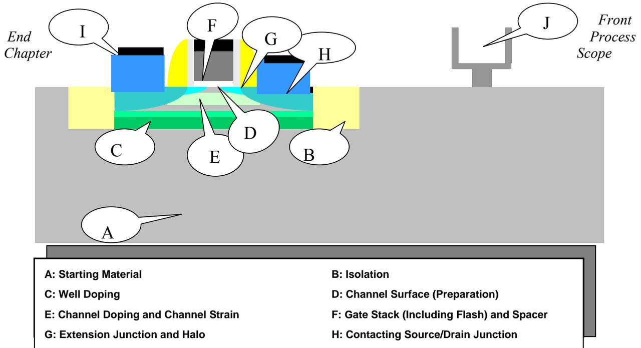
Figure MM12: Front-end processes scope.
