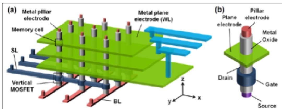
Figure MM8: Schematic view of (a) 3D cross-point architecture using a vertical RRAM cell and (b) a vertical MOSFET transistor as the bit-line selector to enable the random access capability of individual cells in the array [13].
