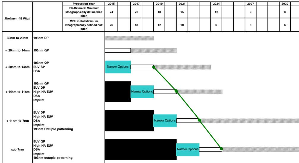
Figure MM13: DRAM critical and MPU metal level potential solutions.
