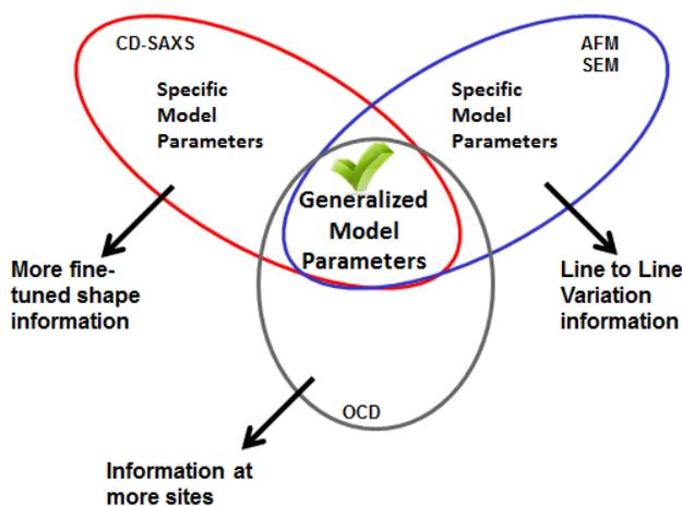
Figure MM17: Conceptual diagram of hybrid metrology. Different instruments provide specific model parameters that are used in a generalized model of the measurement. The arrows indicate specific information from different instruments. Figure courtesy of Richard Silver – NIST.
