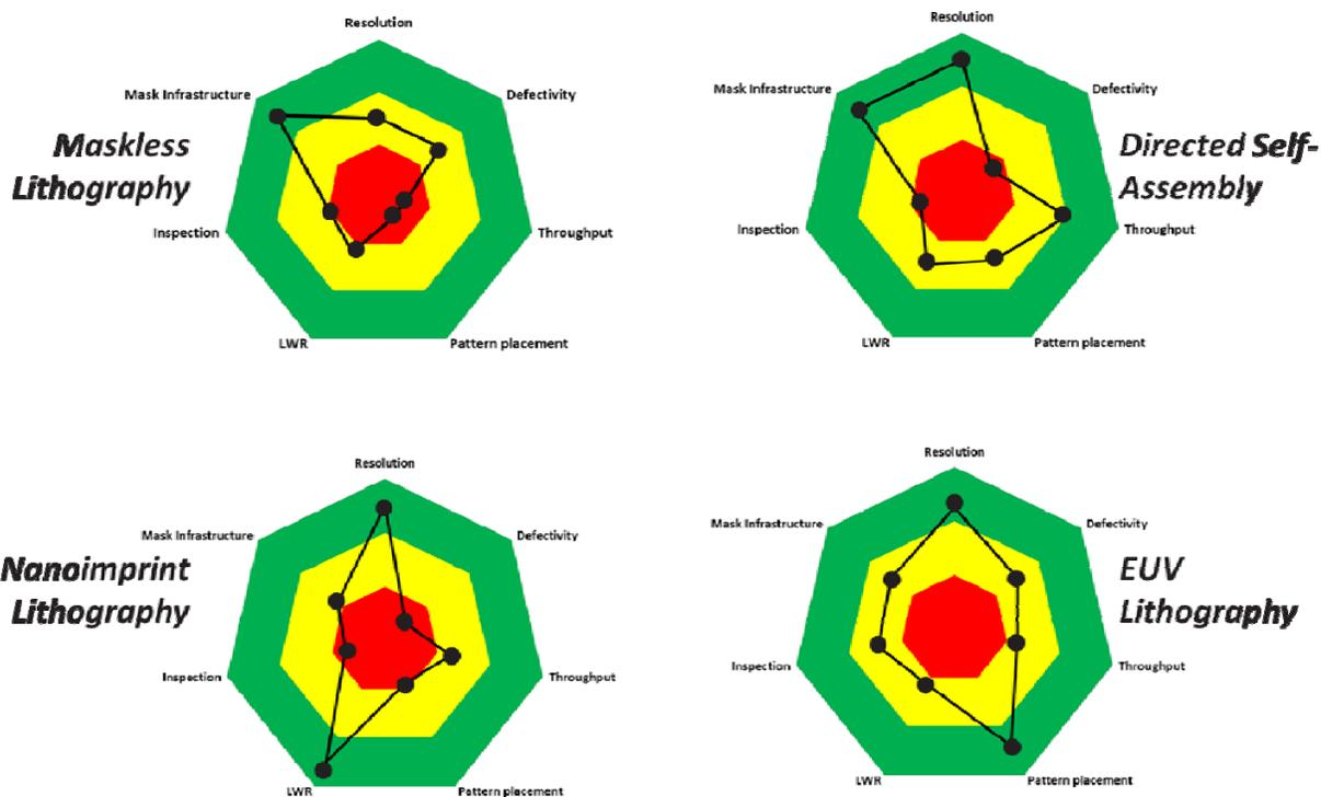
Figure MM15: Radar charts comparing possible alternative to multiple patterning.
