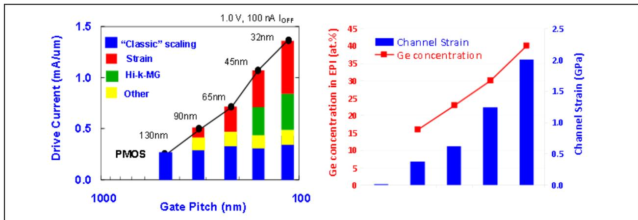
Figure MM5: Impact of strain engineering on device performance [19].
