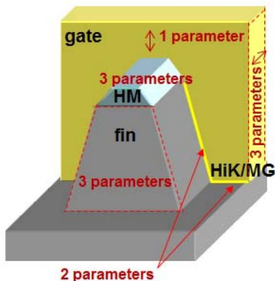
Figure MM16: Complex structures such as finFETs require 3D metrology. To obtain a full 3D profile of the feature above, measurements such as fin CD, height, sidewall angle and roughness, and film thickness are needed. Figure courtesy of Benjamin Bunday, SEMATECH.
