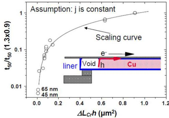
Figure MM9: Experiment and model of lifetime scaling versus interconnect geometry.
