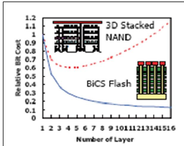
Figure MM6: Comparison of bit cost between stacking of layers of completed NAND devices and making all devices in every layer at once [1].
