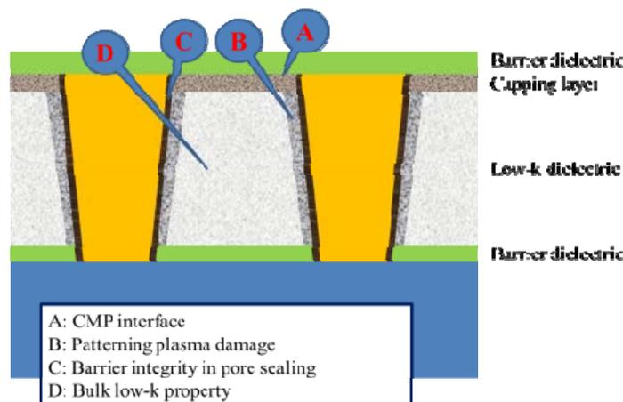
Figure MM11: Degradation paths in low-k damascene structure.
