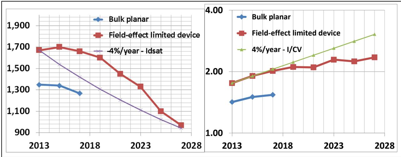
Figure MM2:(left) Idsat (uA/um) and (right) I/CV (ps) scaling trend from the ITRS 2013 edition for bulk planar and field-effect limited devices (e.g. finFET).
