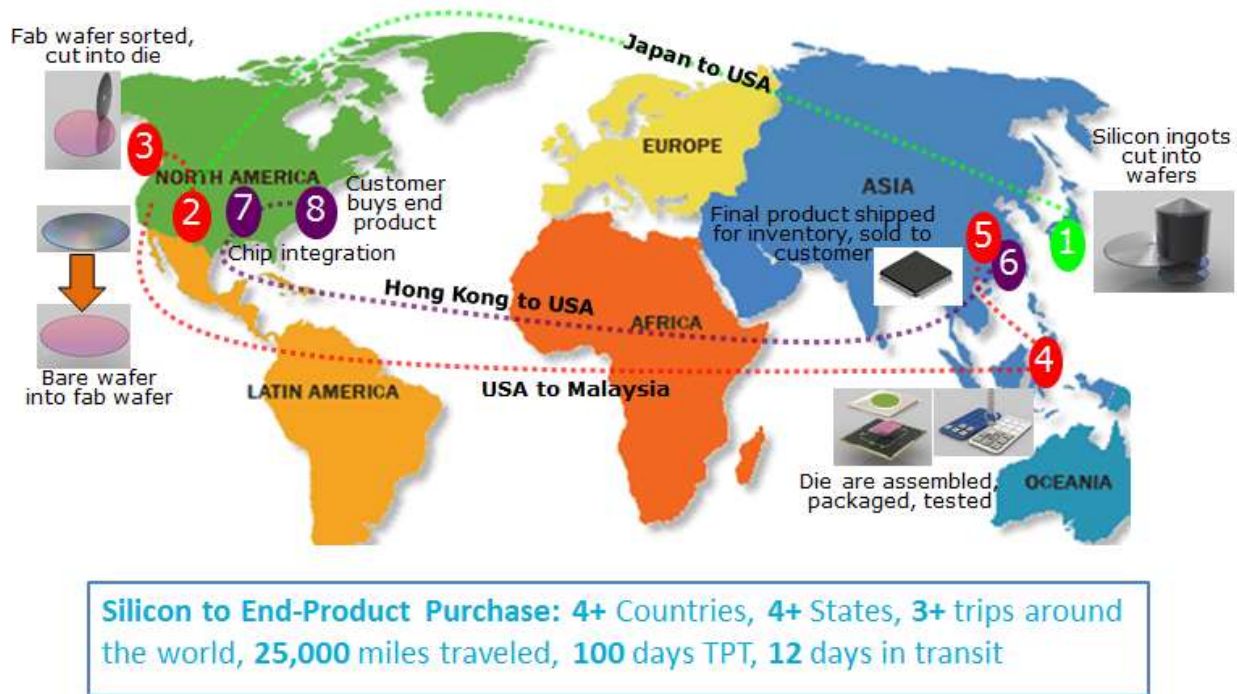
Figure 2: Example of Semiconductor Product Global Manufacturing Process
