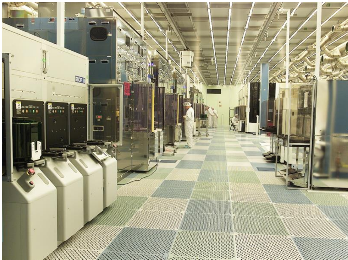
Figure 1. Photo of typical 300mm wafer manufacturing cleanroom.
