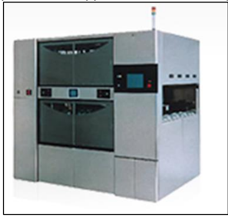
Figure 5. Typical coater/developer tool in which NMP solvent pre-wet and NMP containing photoresist application would take place.
