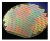
The circuit elements (transistors, resistors, and capacitors) are built in layers on the silicon wafer to produce thousands of electronic devices at tiny sizes, which together function as integrated circuits (ICs). At this stage of the manufacturing process, referred to as "fabrication", the function of the die is fixed or determined. That is, the die is either "multipurpose" or "application specific."
