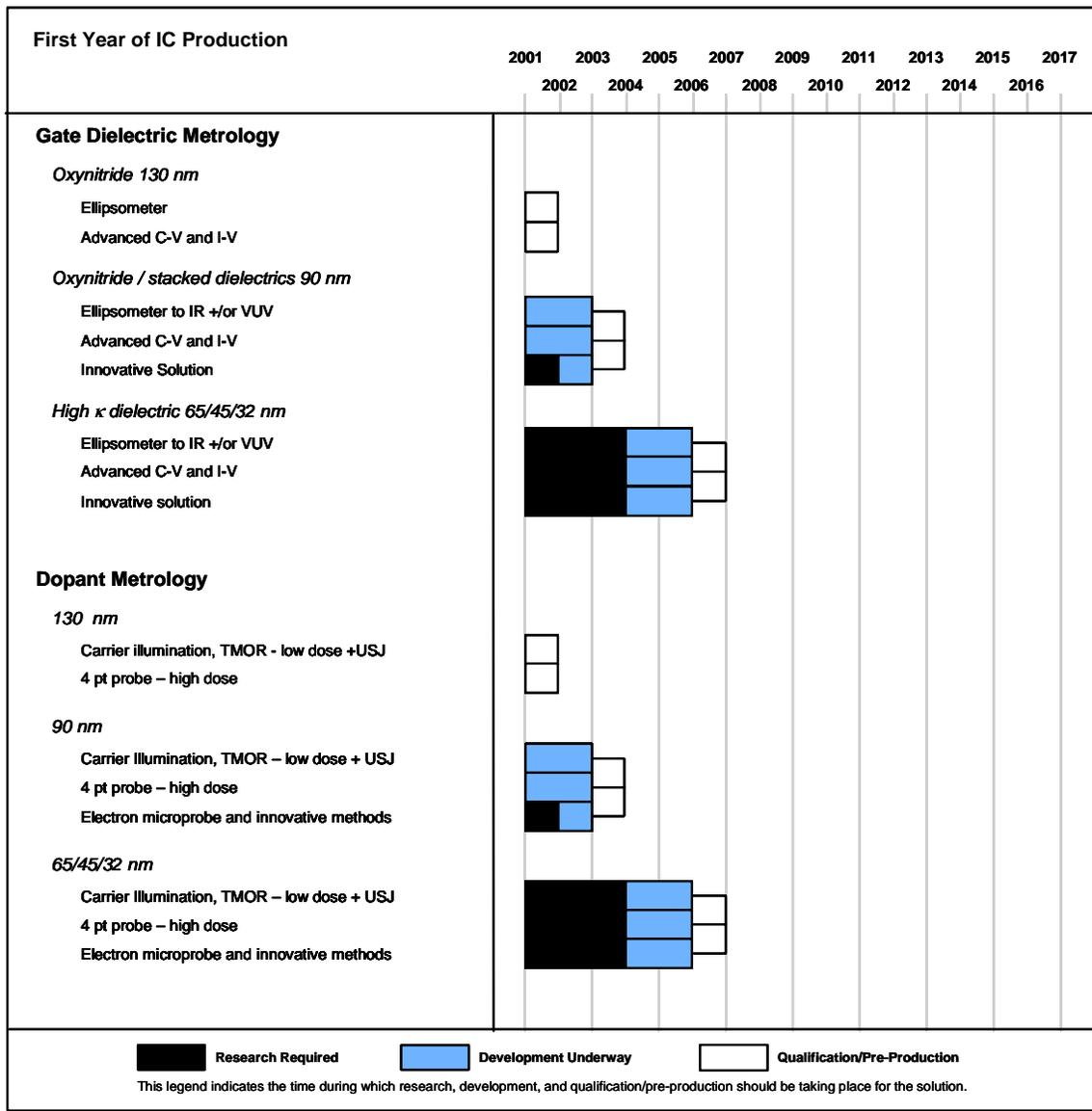
Figure 62 Front End Processes Metrology Potential Solutions
