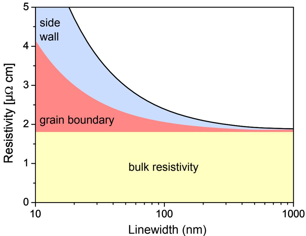
Figure 68 Cu Resistivity
