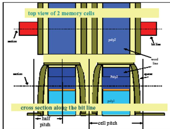
Figure FEP8 Minimum Feature Size of NAND Flash Memory
