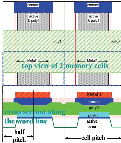
Figure FEP9 Minimum Feature Size of NOR Flash Memory
