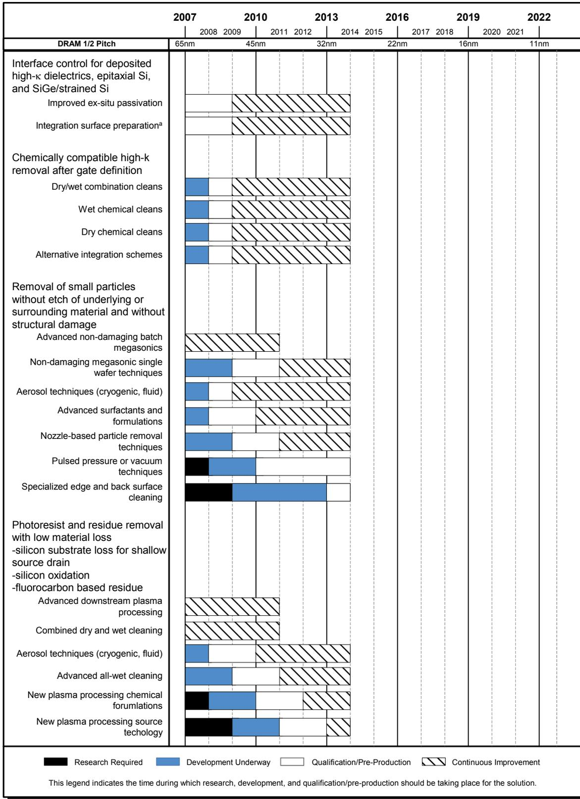
a) Integrated Surface Preparation techniques include various techniques that can be coupled to the deposition chamber and allow processing to continue with minimal exposure to the atmosphere. This includes, but is not limited to, UV-based cleaning, gas phase techniques, and single wafer wet techniques.
