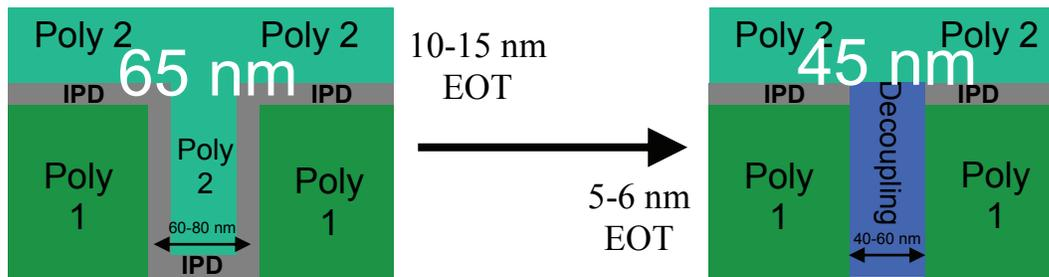
Figure FEP10 Flash Memory Interpoly Dielectric Thickness Scaling at 45 nm
