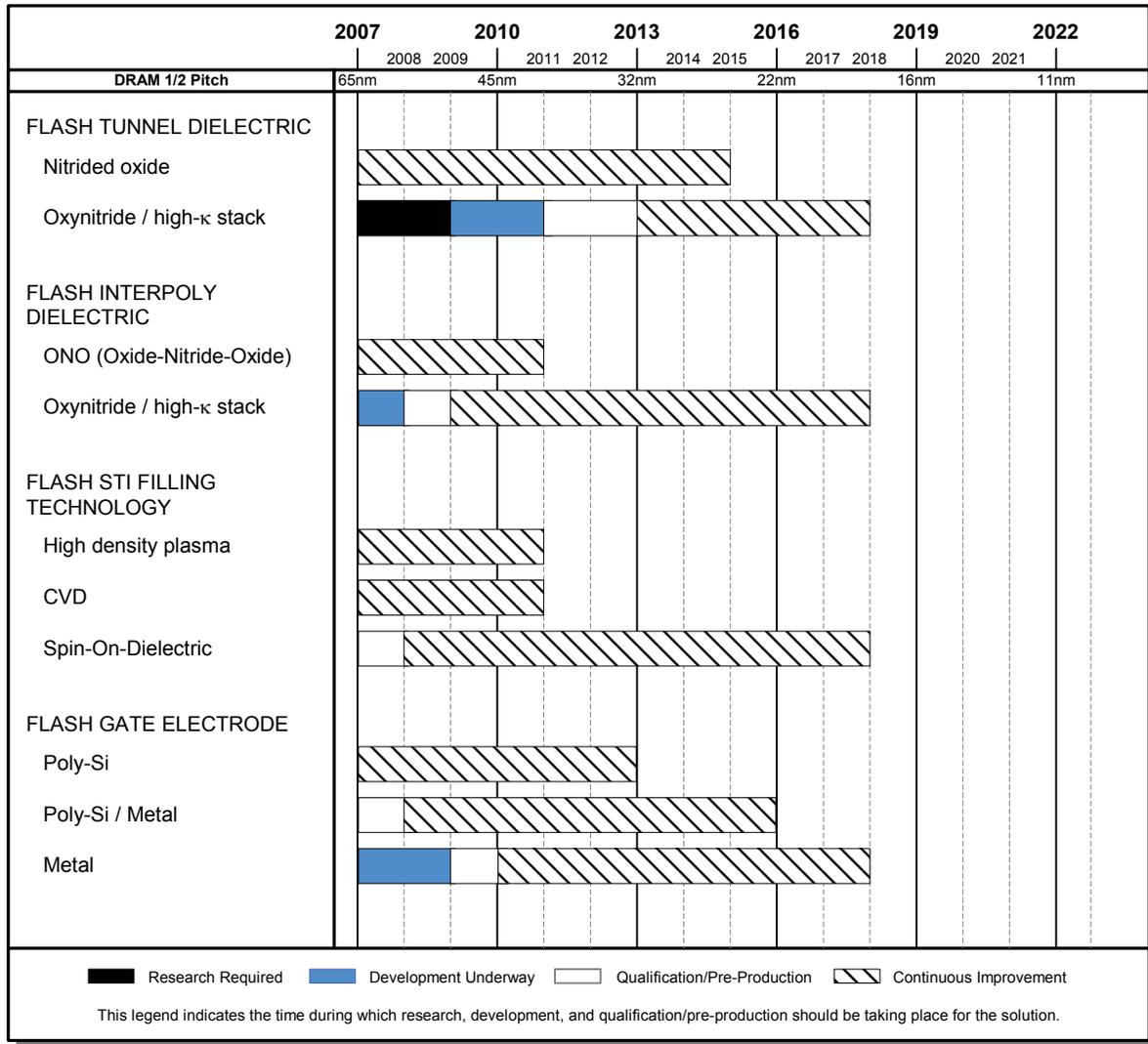
Figure FEP13 Flash Non-Volatile Memory Floating Gate Potential Solutions
