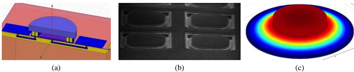
*Figure MEMS10 (a) Schematic cross-section of a capacitive micromachined ultrasound transducer (cMUT), (b) SEM detail of four dual thickness cMUT cells from a 2D array of acoustic pixels, and (c) COMSOL simulation of the first eigenmode of a dual thickness cMUT cell.*
