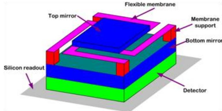
Figure MEMS8 A MEMS Narrow Band Tunable Filter.<sup>16</sup>
