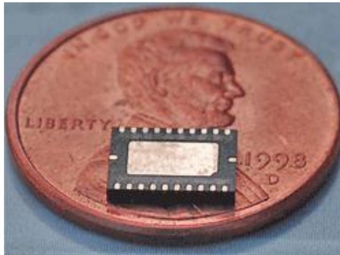
*Figure MEMS7                      The Si Time SiT9104 provides six single-ended clock outputs, two from each PLL, which can operate at up to 220 MHz. Each PLL and associated pair of clock outputs can be driven by independent voltage supplies (1.8, 2.5, 2.8 or 3.3 V), and each output pair on the differential output SiT9103 can be configured to one of three signaling levels, LVPECL, LVDS or CML.<sup>6</sup>*
