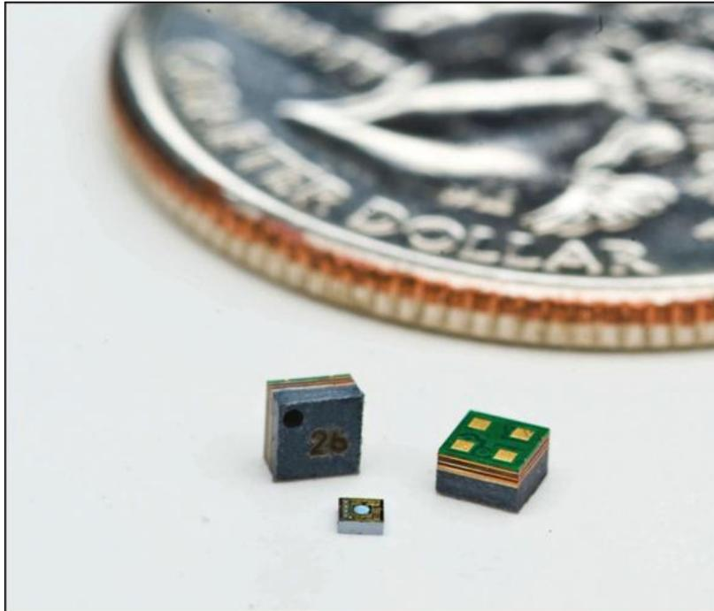
*Figure MEMS6 CMOS MEMS Microphone Die and Packaged Microphones<sup>5</sup>*
