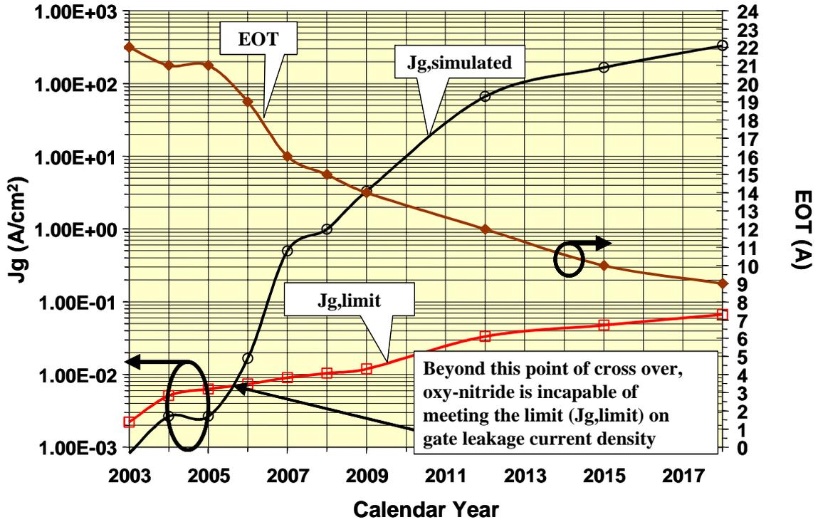
Figure 23 LSTP Logic Scaling-up of Gate Leakage Current Density Limit and of Simulated Gate Leakage due to Direct Tunneling
