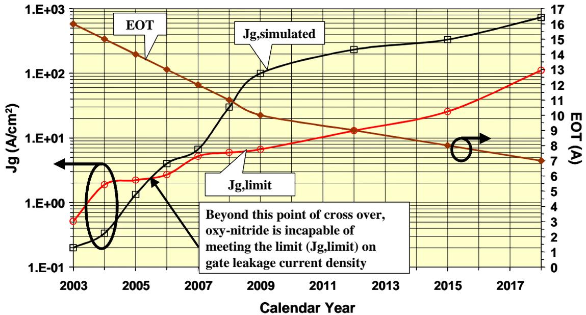
Figure 24 LOP Logic Scaling-up of Gate Leakage Current Density Limit and of Simulated Gate Leakage due to Direct Tunneling
