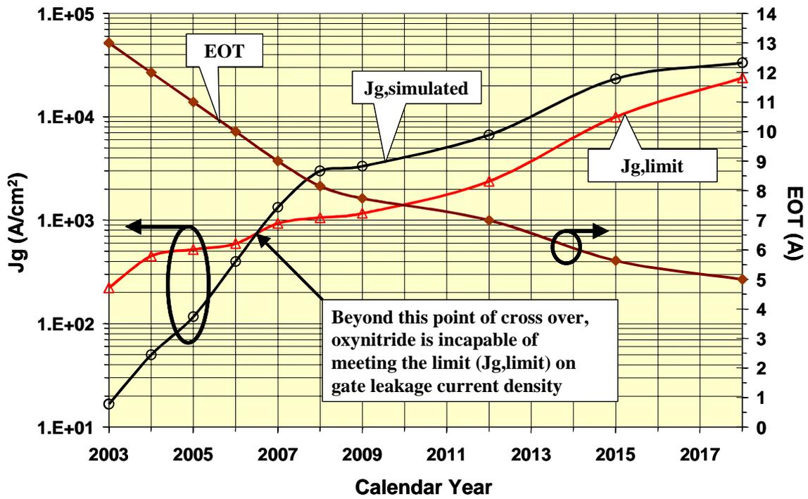
Figure 25 High-performance Logic Scaling-up of Gate Leakage Current Density Limit and of Simulated Gate Leakage due to Direct Tunneling
