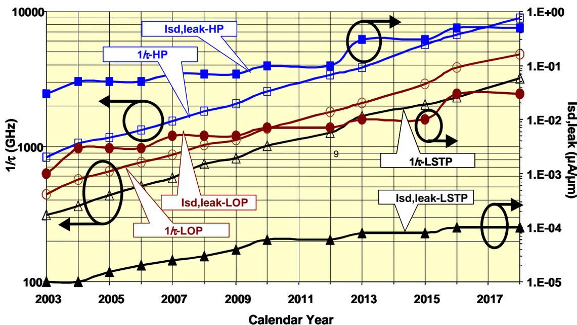
*Figure 22*  $1/\tau$  and  $I_{sd,leak}$  Scaling for High-performance (HP), Low-operating Power, and Low-standby Power Logic
