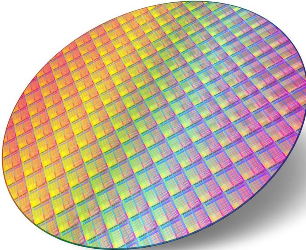
Figure 1: A finished silicon wafer. Each square is an individual semiconductor device.
