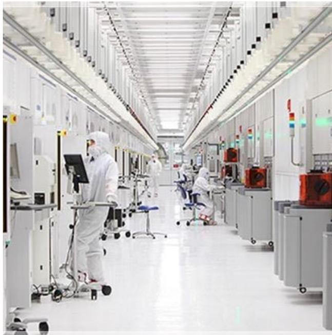
Figure 4. Robotic system moves wafers inside enclosed containers (FOUPs).
