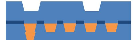
Etch contrast provides self-alignment
