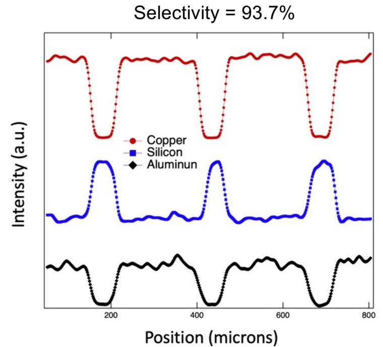
**TMPS SMI blocks at least 4 nm ALD on  $\text{SiO}_2$ , while allowing growth on Cu.**
