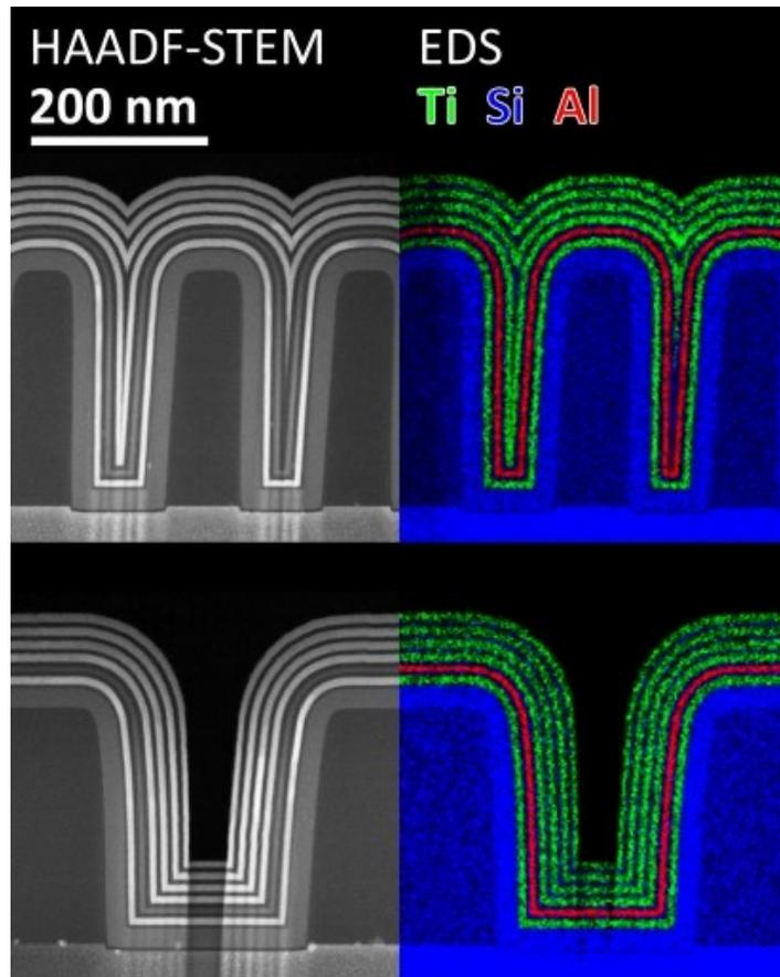
Cross-sectional HAADF-STEM images and corresponding EDS maps, showing a stack of alternating TiO<sub>2</sub> and SiO<sub>2</sub> layers and a single layer of Al<sub>2</sub>O<sub>3</sub>, all grown by plasma ALD on nanoscale trench structures.
