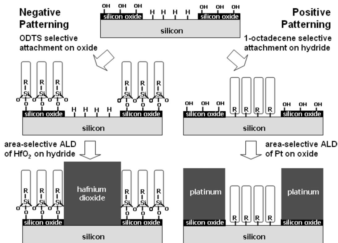
Motivated by transistor high k gate stack (FEOL)
