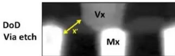
TEM EDS images of DoD deposition showing high selectivity to deposition on oxide, with SAM blocking dep on metal
