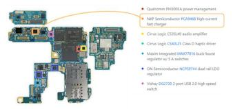
Enabled Efficient Mobile Fast Charging possible with effective Thermal Management
